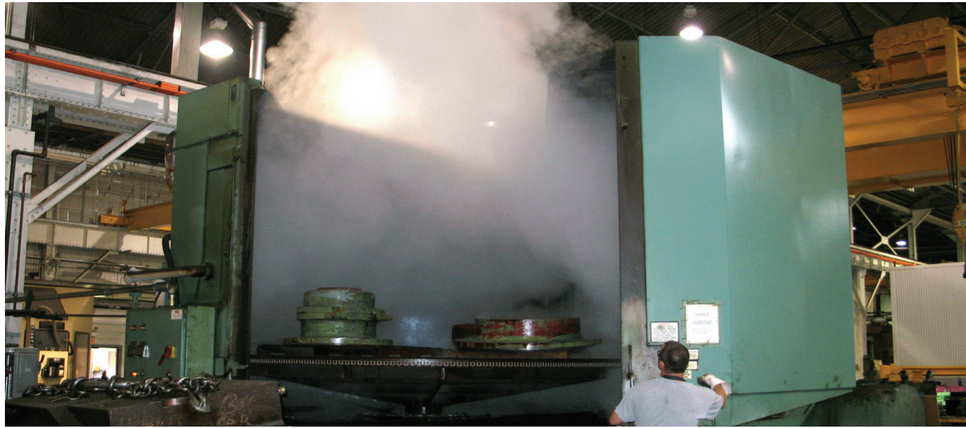
Components being cleaned prior to inspection in an industrial parts washer in Warren, OH, USA
